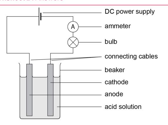
**Anode** – this is the positive electrode to which negative ions migrate during electrolysis
