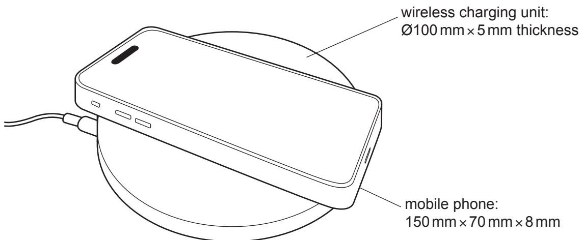
Design a mobile phone charging station for a hotel room that incorporates the wireless charging unit shown. The charging station must be wall-mounted and be clearly identified as a place where a mobile phone can be charged.
