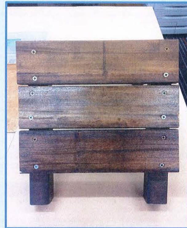
Top layer - Outdoor furniture oil Middle - Shellac Bottom - Outdoor wood stain
