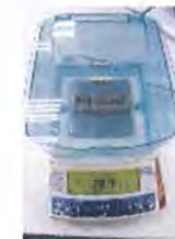
Mass is measured using Electronic Balance.
