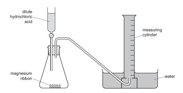
30 cm<sup>3</sup> of dilute hydrochloric acid was added to the conical flask containing magnesium ribbon.
