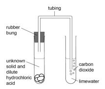
(e) The limewater will go cloudy as the CO<sub>2</sub> is bubbled through it.
