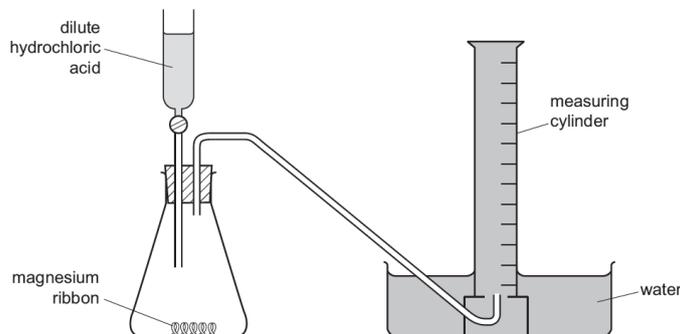
30 cm<sup>3</sup> of dilute hydrochloric acid was added to the conical flask containing magnesium ribbon.
