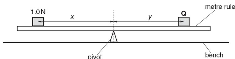
A 1.0 N load was placed on the metre rule so that its centre was at the 20.0 cm mark. The distance  $x$  between the 20.0 cm mark and the pivot was recorded. Load **Q** was placed on the metre rule and its position adjusted so that the metre rule is as near as possible to being balanced. The distance  $y$  between the centre of load **Q** and the pivot was recorded.
