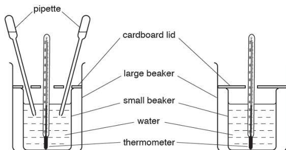
They placed hot water in two small beakers and stood each one in a large beaker. One beaker had 'ears' and one beaker did not. The 'ears' are represented by two small dropping pipettes. The pipettes were continuously squeezed and released throughout the experiment so that water continuously moves out of and into the pipettes.
